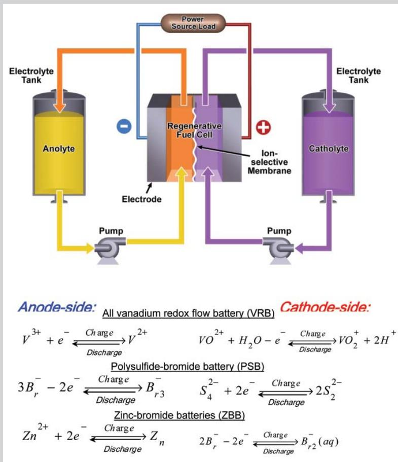
Figure 3. A schematic of a redox flow battery and selected redox chemistries.
