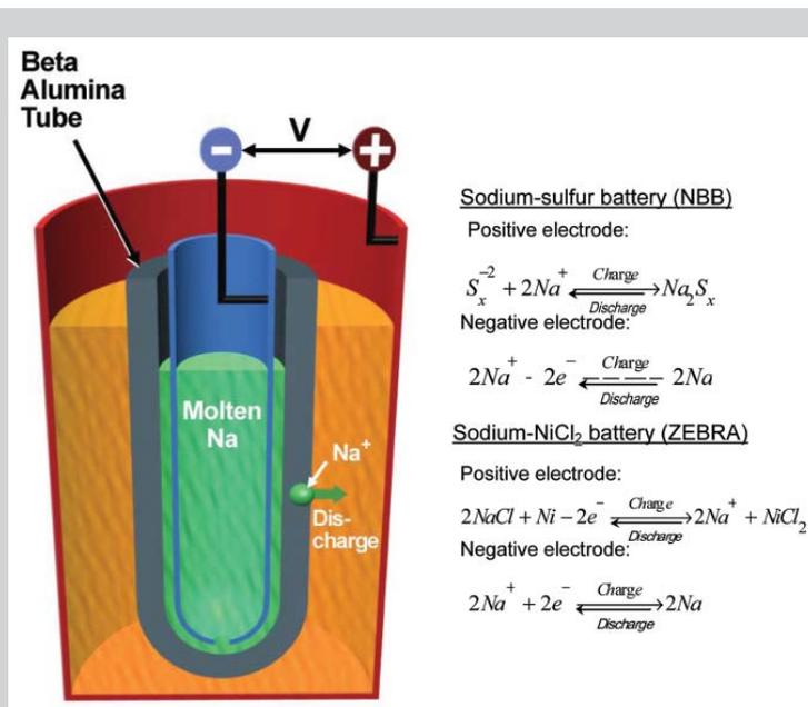
Figure 4. Single-cell and tubular design of a sodium-beta battery and electrode reactions.
