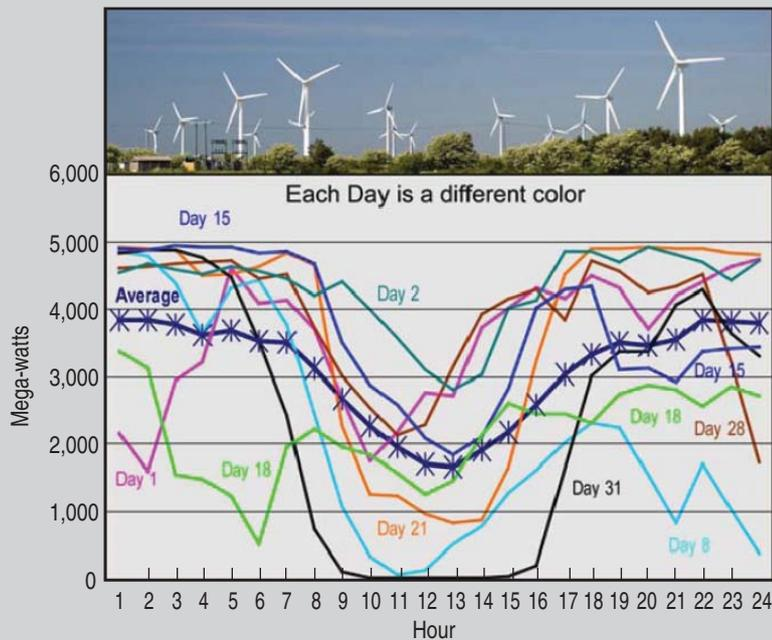
Figure 1. Daily profiles of wind power projected by 7x output in April 2005 for the year 2011 in Tehachapi, California. (Courtesy of ISO California.)
