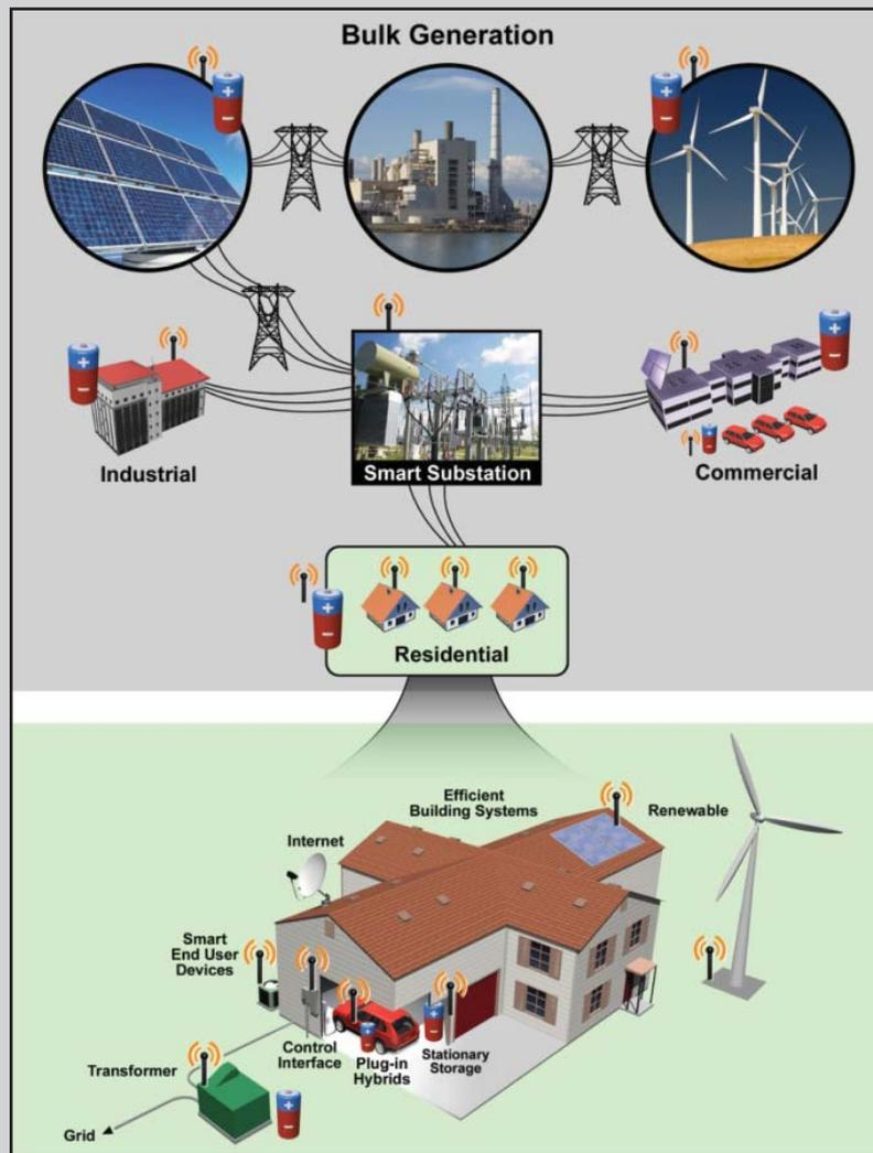
Figure 2. A schematic of applications of electricity storage for generation, transmission, distribution and end uses, and a future smart grid that integrates with intermittent renewables and plug-in hybrid vehicles through two-way digital communications between loads and generation or distribution grids.
