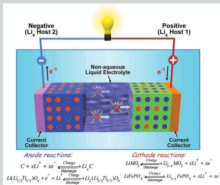
Figure 5. A schematic of a lithium-ion battery cell in which, during discharge, Li<sup>+</sup> ions migrate through the electrolyte and electrons flow through the external circuit, both moving from the anode (– electrode) to the cathode (+ electrode), along with selected electrode reactions.
